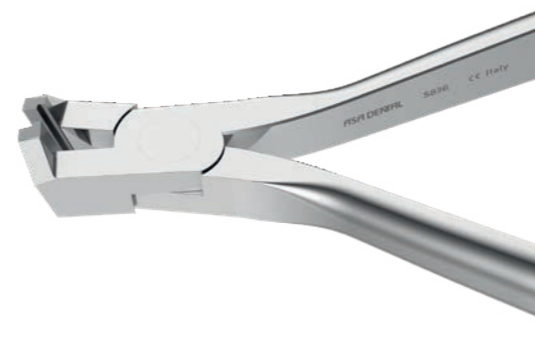
distal end cutter 5836 Distal end cutter with safety hold designed to cut hard wires and hold the loose distal end, preventing damage to oral tissue. Wire size: rectangular max. 0.56 mm x 0.7 mm (0.022" x 0.028") round max. 0.5 mm (0.020")
