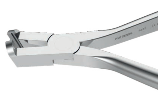
micro distal end cutter 5837 Distal end cutter with safety hold designed to cut hard wires and hold the loose distal end, preventing damage to oral tissue. Wire size: rectangular max. 0.56 mm x 0.7 mm (0.022" x 0.028") round max. 0.5 mm (0.020")
