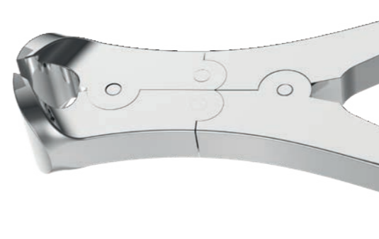
wire cutter <= 1.2 mm 5880-3TC Distal end cutter designed to cut wire pins and ligature wires, strong enough to bend wire ends after distal cutting. With tungsten carbide inserts. Wire size: max. 1.2 mm (0.044")
